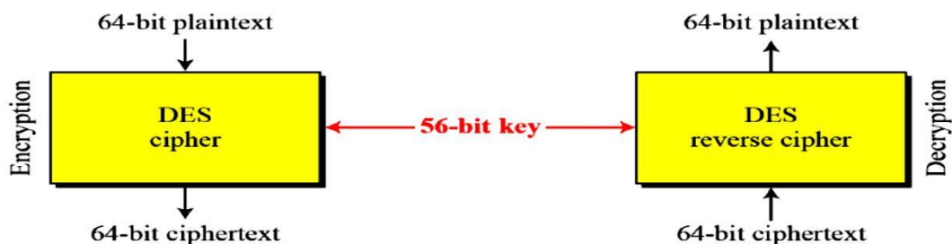
Encryption and decryption with DES
