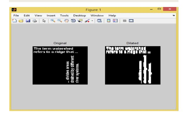
Example to apply a dilate operation on grayscale image with a rolling ball structuring element:
