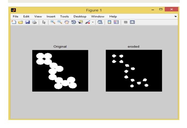
Example to apply an erode operation on a grayscale image with a ball structuring element:
